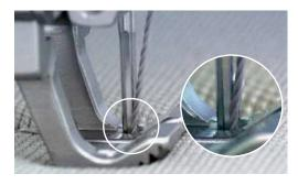
Sewing of very dense or very hard materials leads to crushing of the thread between the sewing fabric and the scarf edge during the needle down stroke.
