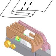
Differential feed dog system Left and Right differential feeding effects to prevent puckering for stretch Jeans
