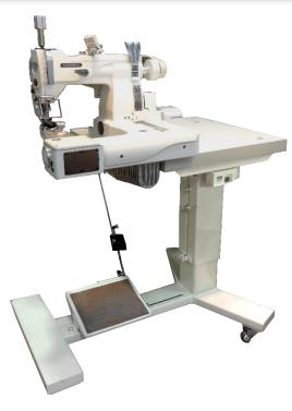
3 needle, feed-off the arm, double chain stitch for heavy duty material with differential feeding mechanism
