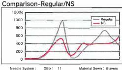
Penetrating Depth: 15mm Penetrating Speed: 250mm/min
