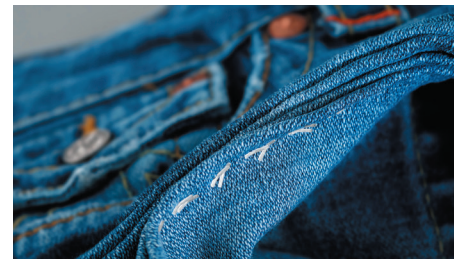
Denim whiskering process using Plastic Staple fasteners
