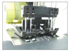
Model 3324 Closeup of the four needles
