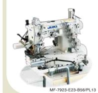
This model is best suited for sewing elastic bands on briefs. E22 is opened / closed with the knee lever and E23 is opened / closed with the knee switch. The machine comes provided as standard with a tension roller to smoothly sew elastic bands on different-sized garment bodies. The machine flexibly adapts to varying elasticities due to its soft seams
