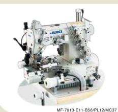
This model is best suited to endless flat elastic band sewing processes for briefs, boxer briefs etc. The right hand fabric trimmer trims the fabric, even at a multi-layered joined part, to produce a beautiful finish with the seam and fabric edge aligned with consistency. Cloth cutting knife can be detached with one touch operation in case of sewing without using the knife.
