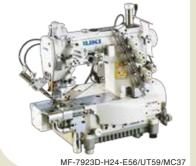
The machine is best-suited for the hemming of stretchy new material such as T-shirts, underwear and sportswear, etc. The machine produces seams with no semi-cylindrical swells by performing sewing while making the feeding lengths of the right and left needle threads equal. The sliding presser foot prevents the material hem from twisting during sewing and further eliminates oblique-feeding of the material in terms of its texture.
