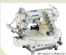
The machine can be used for the hemming process of the sleeves and bottoms of T-shirts and for the covering process for sportswear and knitwear.
