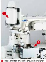
2 Thread trimmer drive mechanism magnet
