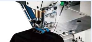
The machine is provided with the digital type top feed mechanism
