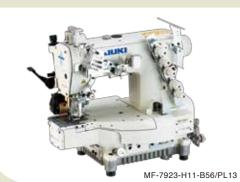
This model is best suited to elastic-band welting for swimwear, briefs, etc. It welts the elastic band which has been overlocked on the garment body.
