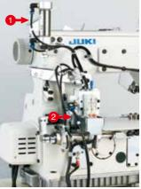
Presser lifter drive mechanism air cylinder 2 Thread trimmer drive mechanism air cylinder
